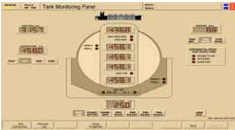
MD 506 tank monitoring panel
