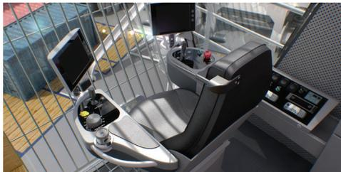
A sound insulated state-of-the-art cabin houses the operator's chair with redundant touch screens, camera monitors, a writing desk and a co-pilot chair. Heating and air conditioning allows the operator to work comfortably and efficiently in all climates.
