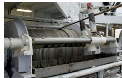
Winch upgrade with electric spooling gear
