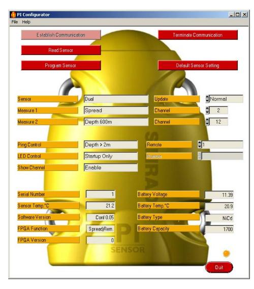
use in the sensors will also require this combination. Older versions of the **PI Configurator** will not work on the latest sensors. The old types of interface cables will also prove unoperational on the latest sensor electronics.
