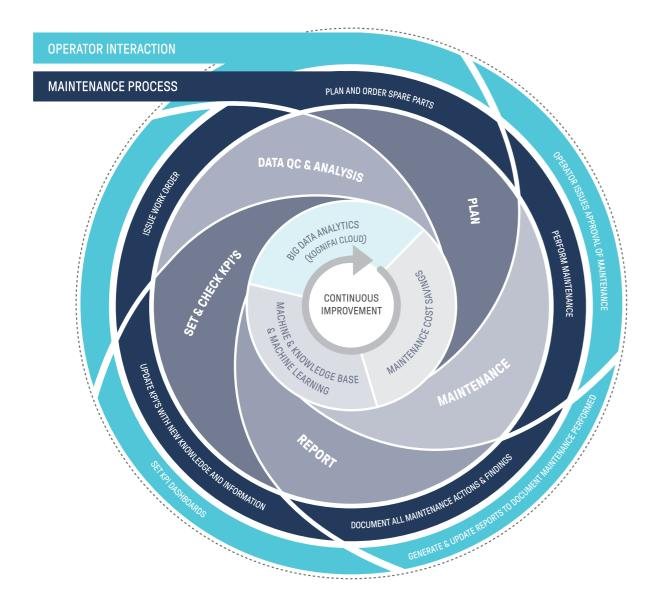
The KONGSBERG CBM Decision Support Wheel illustrates the workflow that shapes a modern Condition Based Maintenance strategy. By using big data analytics, the condition monitoring system detects abnormalities which in turn initiates work orders. The ability to plan and conduct 'in-time' maintenance leads to reduced cost. Documentation of all maintenance actions and findings increases process knowledge, leading to continuous improvement of your analysis.
