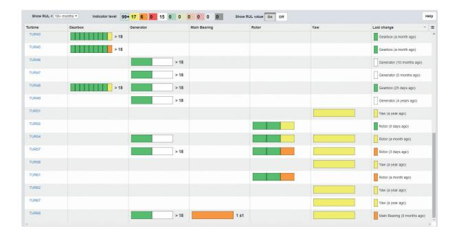
The TUR68 asset shows that an alarm was raised 9 months ago for the Main Bearing. The RuL is predicted to 1 months +/- 1 month. Replacing the bearing is critical.
