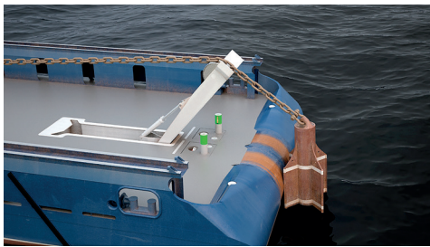
A-LARS in max position, anchor in water
