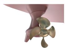
The streamlined leg and skeg recover swirl energy from the slipstream of the pulling propeller, raising the overall propulsive efficiency because this otherwise wasted energy is converted to a forward force on the thruster leg.
