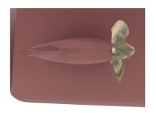
The flow of water to a pulling propeller is only determined by the hull, and it is possible to obtain a more homogeneous inflow to the propeller in this type of thruster. More uniform inflow is decisive for reducing unsteady cavitation, and thereby cutting down propeller induced noise and vibration and reducing oscillations in shaft torque.
