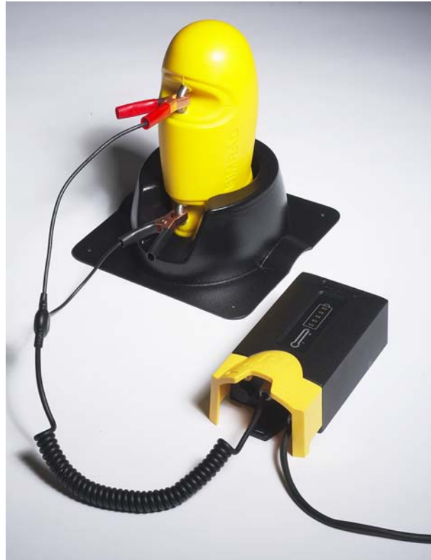
Figure 24 The PI Charger set up to charge a PI sensor
