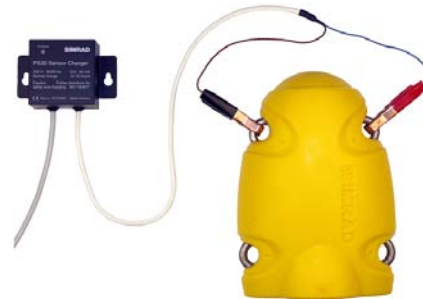
Figure 28 The PS Charger set up to charge a sensor
