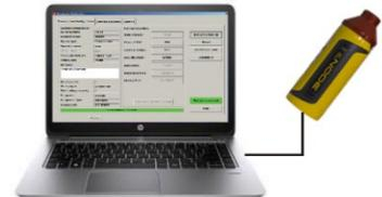
**Note:** A cNODE MiniS transponder (not included) is required to be connected to the PC via the supplied serial cable and act as a transducer/transceiver to run acoustic tests to all cNODE transponder types.
