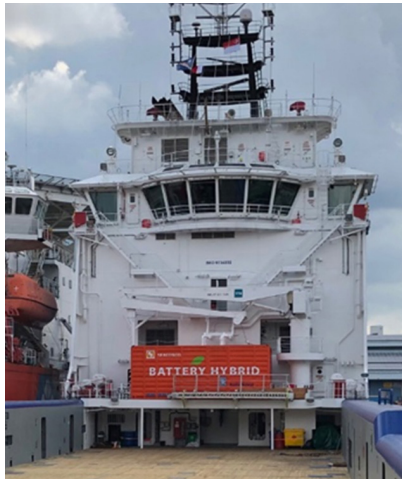
Figure 2 - Example of Deckhouse installed on vessel
