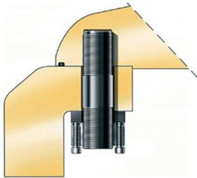
A unique type of bolt is used to install the blades on the hub. The bolts can be tightened using light hand tools from inside the hub.
