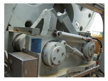
A full capacity chain stopper dimensioned for the MBL of the chain is provided. The design is fail-safe and the stopper also have load measurement incorporated.
