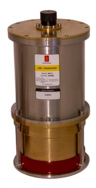
$\mu$ PAP is a portable and compact acoustic positioning system for tracking ROVs, tow fish, divers or other subsea objects at several thousand metres range. The transducers are mounted on a pole for installation over-the-side or through a ship's moon pool. The system is easy to install on ships or other surface units and comes with a wide range of transponder channels and cNODE® transponder models for depths down to 4000 metres.
