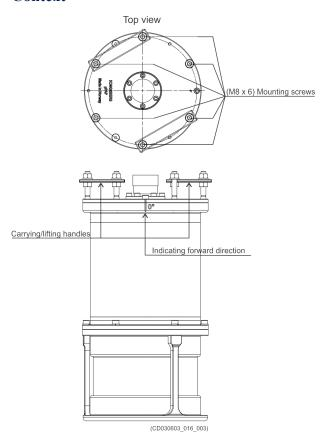
The transducer is mounted on the ship's arrangement for the transducer. This may be on a pole lowered through a moon pool or a hull unit.
