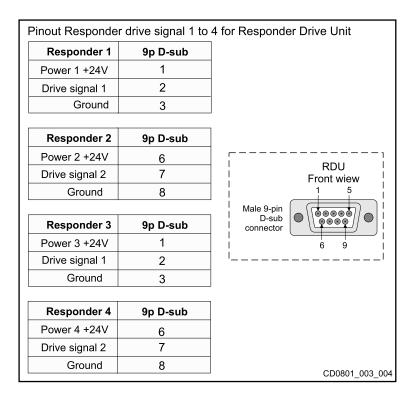
Terminate the responder trigger signal cables as illustrated with D-sub connectors.
