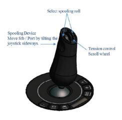
• Operation of spooling gears
