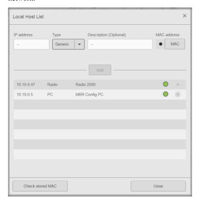
7 Type the IP address of the equipment you want to connect. Select type of equipment from the **Type** list. Type a description of the equipment for identification purposes.
