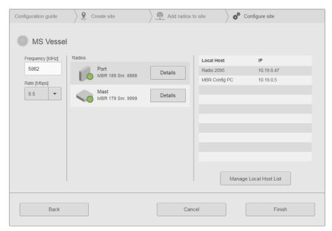
5 Type the radio frequency. Select the data rate for the radio site from the **Rate** list.
