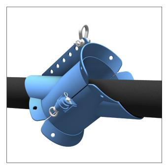
The simple and lightweight, yet robust construction of the corer clamps with minimal moving parts, allows easy handling and flexible positioning along the corer barrel, and keeps maintenance requirements to a minimum.
