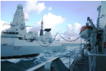
RAS & FAS Transfer
