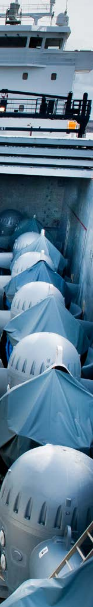
The largest order for UUC underwater mountable thrusters to date was for the innovative Allseas heavy lift vessel Pioneering Spirit . The picture shows the 13 thrusters being loaded for the voyage to the buildyard in Korea
