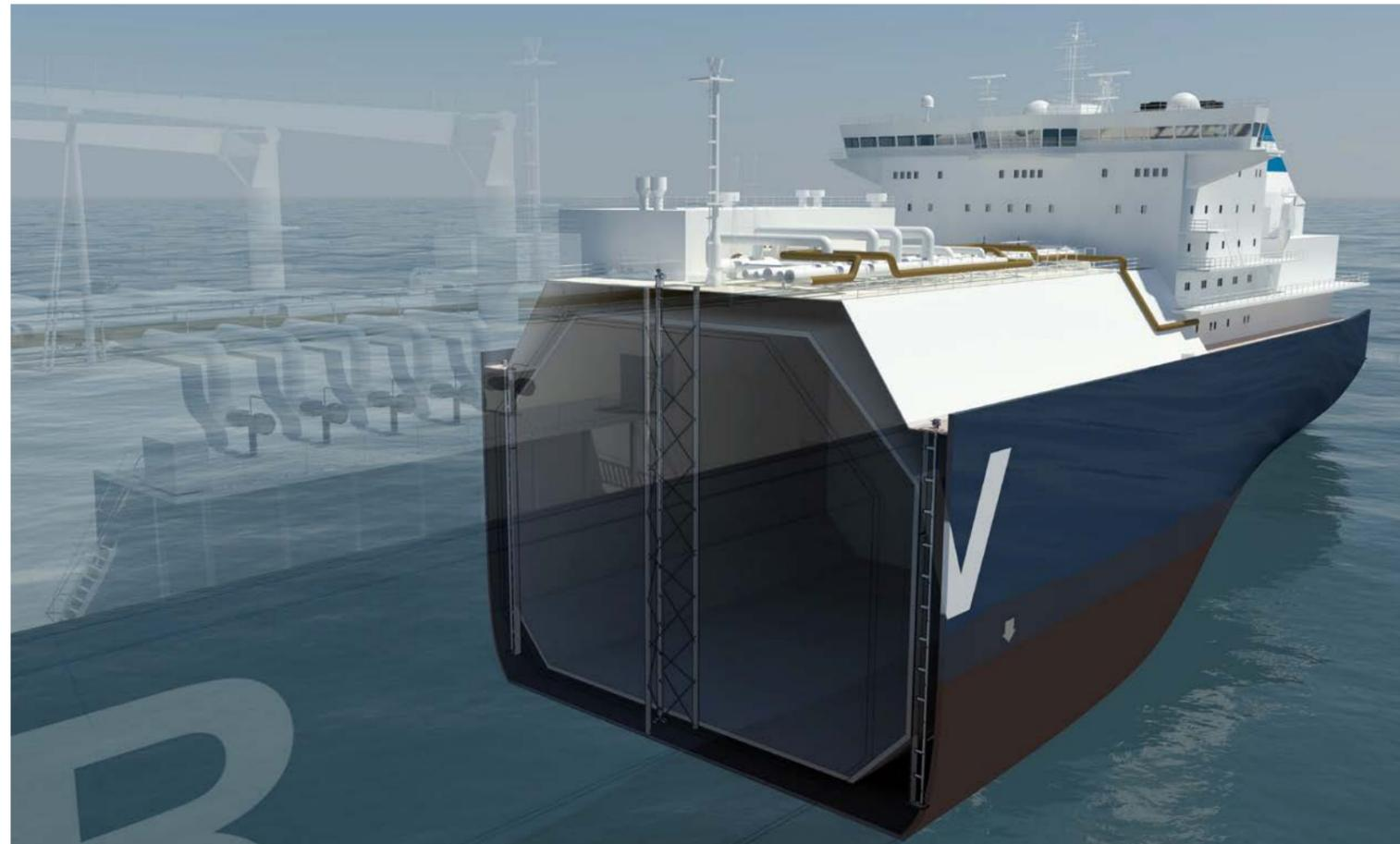
Each pipe section is supplied with flanges prepared with reference markers. The liquid level and the markers are measured simultaneously, hence the system automatically verifies itself at every measurement. By careful calibration of the pipe section lengths before installation, the position of the markers are recorded and stored in the system. By comparing the liquid echo with the reference marker echo, a continuous auto-calibration of the measurement is done.
