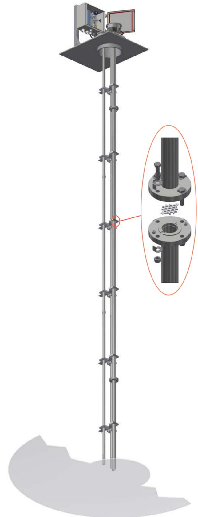
Figure 7: Standpipe installation with marker for auto-calibration by AutroCAL® (example)
