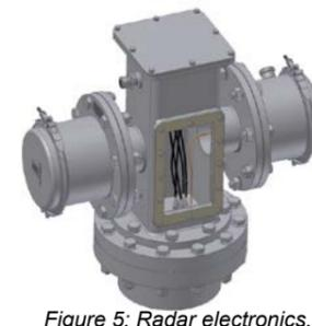
Figure 5: Radar electronics, CTUs and temperature sensor installation (example)
