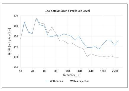
Full scale Sound Pressure Level from measurements of radiated noise in the cavitation tunnel at Kongsberg Hydrodynamic Research Centre for a propeller operating in a non-uniform inflow. Measurements confirms the experience from installations on Naval vessels that underwater broadband noise levels are significantly reduced.
