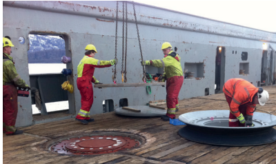
Mounting of rope tensioners at Island Vanguard
