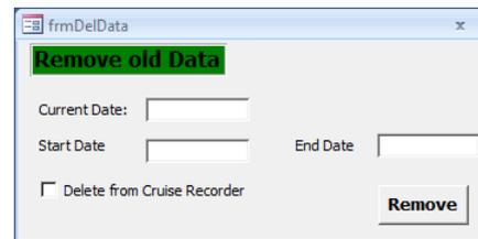
You are only permitted to use a start date and an end date to select the data to be deleted. Both dates are inclusive. The recorded information from all sensors within the defined time period will be removed. You are not able to delete information for specific sensors.
