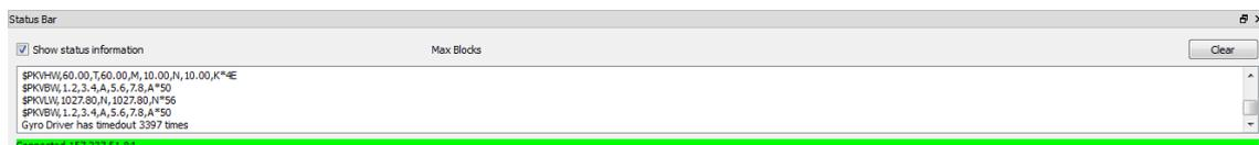
When opened and activated, the text field in the Status Bar provides messages generated by the Sensor Drivers currently in use on the computer. To choose which Sensor Driver to contribute to these messages, check the applicable sensors using one of the status switches at the top of the **Client Manager** dialog.
