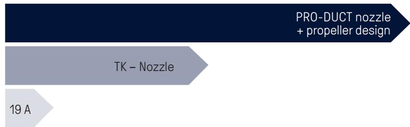
Comparison of received bollard pull per device with the same power
