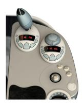
Speed and tension controls on the right arm rest
