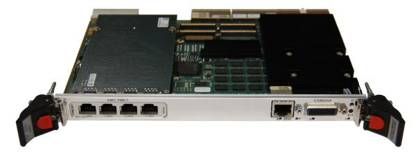
The Concurrent PP B12 is a PC-compatible high functionality Compact PCI (cPCI) board used by the EM 304 Processing Unit as the Central Processing Unit (CPU).
