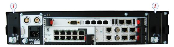
The Processing Unit has two fan units for cooling purposes.
