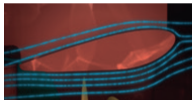
The nozzle profile in a free-running situation. The profile controls water flow to provide a low drag solution.
