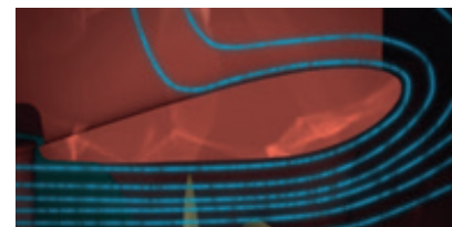
The nozzle profile in towing condition. The shape gives vortex-free flow into and around the nozzle, boosting thrust and improving bollard pull.
