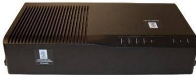
The WBT, the wideband transceiver: Two WBTs, allowing for up to 8 simultaneous depth observations can be used with EA440.
