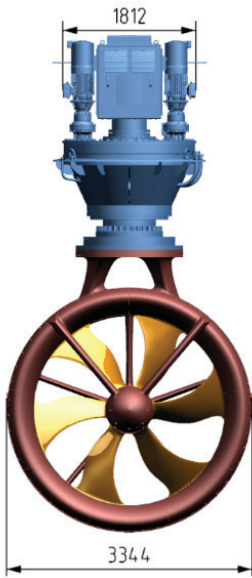
Thruster seen from forward side
