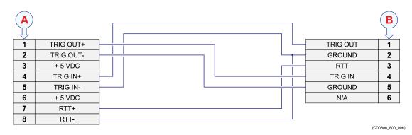
A Connections on the EM 2040 Processing Unit. RJ45 connector
