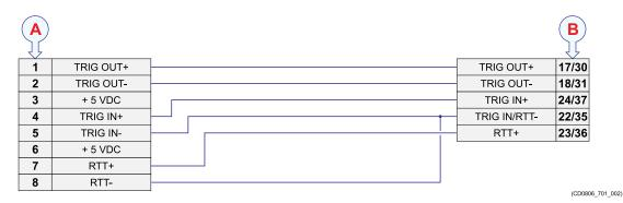
**A** Connections on the EM 2040 Processing Unit. The connector is RJ45 type.
