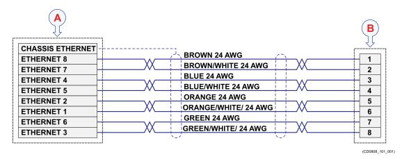
For deliveries before Q2 2011 the cable may be connected according to this diagram:
