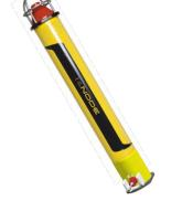
Note: The transponder endcap module can be preconfigured to accept a RS-232 serial input from external instruments like a Paroscientific Digiguartz® pressure sensor or Mesotech 1007/1107D altimeter, etc. The serial endcap module can supply an output voltage of 24 VDC to the external sensor.
