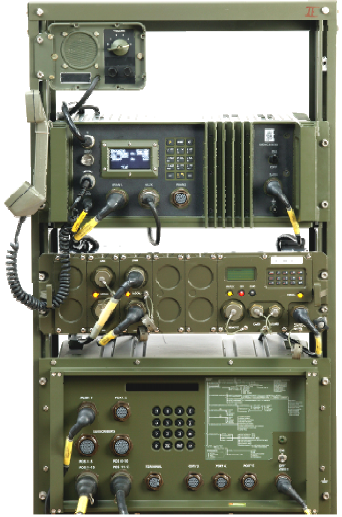
Rack with RL532A, Bulk Encryption Unit CD510 and Multimedia Switch CPX300
