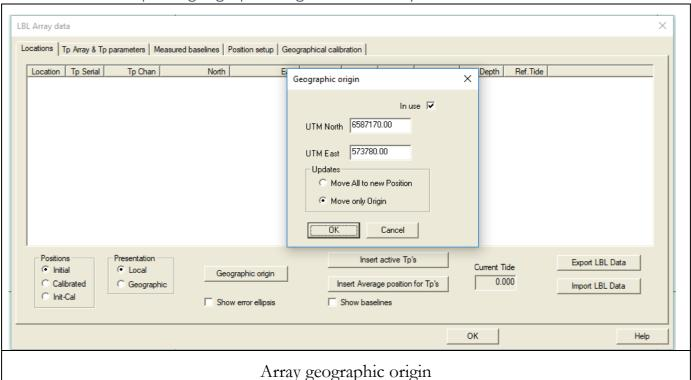
5. Use LBL Array Data, *Insert Average position for Tp's* to set transponder locations. This will suggest the transponder locations established in 3.
