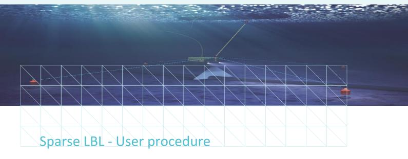
Sparse LBL enables LBL positioning of an ROV using only two cNODE seabed transponders. This function can be combined with HAIN.
