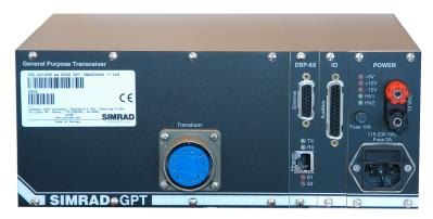
The input power for the General Purpose Transceiver must be kept between 110 and 250 VAC. When installing or moving a GPT, make sure the input power is kept between 110 and 250 VAC.
