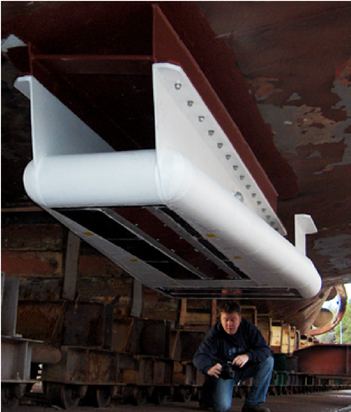
Figure 9 Gondola – 1 x 2 degree system
