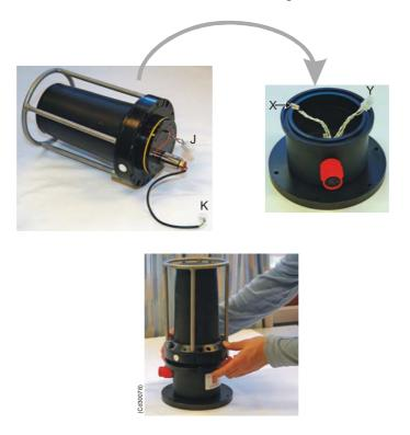
Figure 18 Mounting the split transducer-head 1
