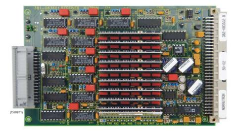
Figure 33 Receiver circuit board
