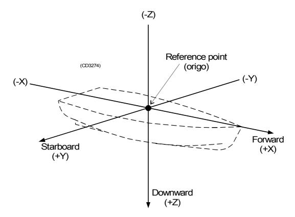
Figure 121 - The Vessel Coordinate system
