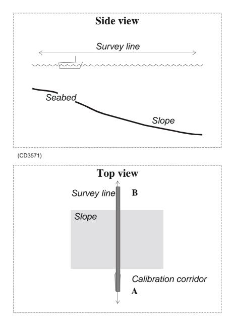
Figure 93 - Pitch offset and time delay calibration procedure
