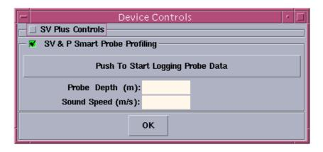
Figure 59 - The **Device controls** dialogue box, SV & P Smart Probe Profiling
