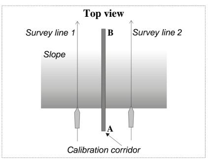
Figure 94 - Heading offset calibration procedure (Alternative 1)
