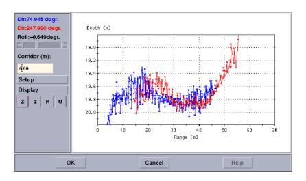
Figure 97 - Calibration profile window for roll calibration
