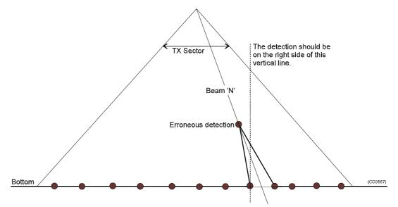
Figure 42 - Slope filter principles
