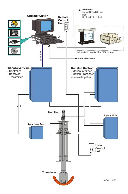
Figure 2 - EM 1002 with hull unit - simplified system diagram
