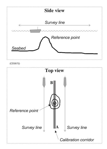
Figure 95 - Heading offset calibration procedure (Alternative 2)
