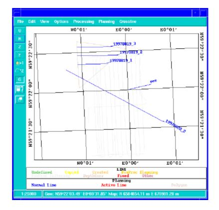
Figure 101 - Survey Display example with survey lines, planned lines and a polygon
