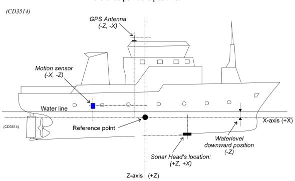
Forward position is defined on the X-axis (refer to the illustration below). Locations further forward than the reference point are positive.
