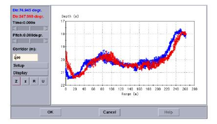
Figure 98 - Calibration profile window for **pitch/time** calibration
