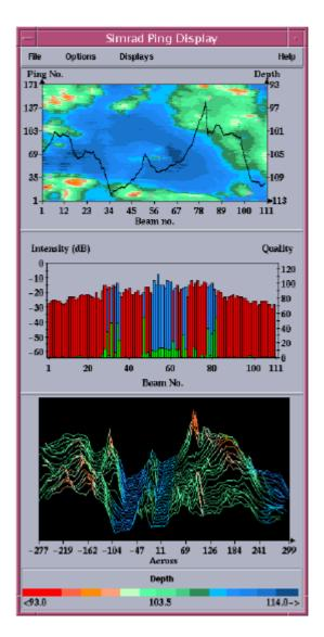
Figure 61 - The Ping Display main window
