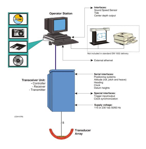
Figure 1 - EM 1002 system diagram
