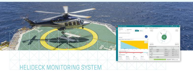
Offshore helicopter operations are carried out in hostile environments. The HMS 300 is designed to measure helideck motion during helicopter pre-landing and on-deck operations to improve flight and passenger safety in these conditions. The system monitors the helidecks acceleration, heave velocity, inclination, roll and pitch together with meteorological data in real-time.
