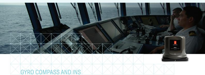
A new family of products with motion sensing and gyro compass functionality is introduced. The MGC R2 product includes three Ring Laser Gyros and three linear accelerometers.
