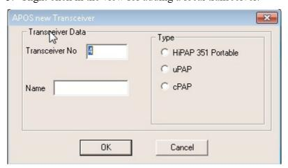
Portable transceivers can be selected between the types shown in the previous dialog box. A local transceiver can also be removed by selecting it and choose Remove transceiver from the menu.
