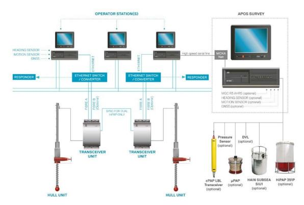
The interface between APOS Survey and onboard APOS is normally a high speed serial line with a galvanic isolated connection.
