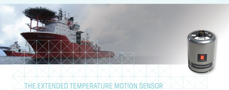
This fifth generation roll, pitch and heave motion sensor is specially designed for use in marine applications that require an extended temperature range. The MRU E is designed to operate at ambient temperatures from -25 to +70 °C and to be installed on open decks, inside cabinets or on bulkheads.
