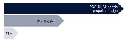
Comparison of received bollard pull per device with the same power
