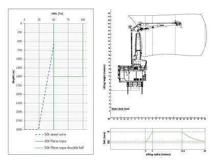
The graphs to right compare the subsea lifting capacity of fibre rope vs. steel wire. Unlike steel wire, fibre rope suffers no depth derating as it has neutral buoyancy. In addition, the fibre rope's twist free construction enables deepwater operations in double fall which effectively doubles the crane's lifting capacity.
