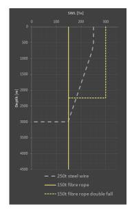
Fibre rope crane 150t vs. 250t steel wire
