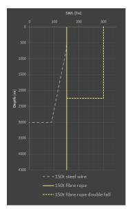
Fibre rope crane 150t vs. 150t steel wire
