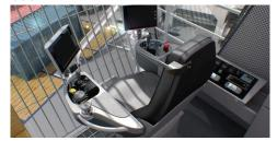
A sound insulated state-of-the-art cabin houses the operator's chair with redundant touch screens, camera monitors, a writing desk and a co-pilot chair. Heating and air conditioning allows the operator to work comfortably and efficiently in all climates.
