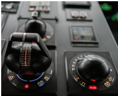
Mcon control system
