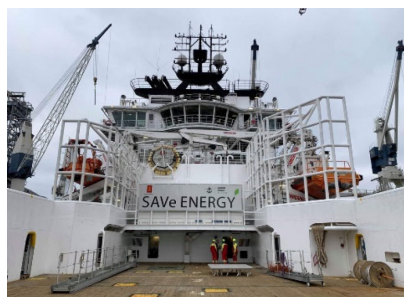
Figure 2 - Example of Deckhouse installed on vessel
