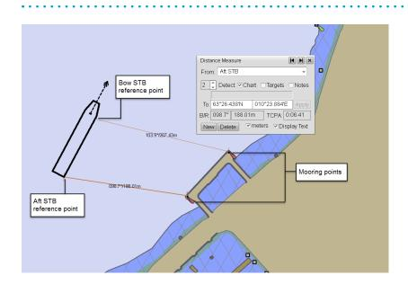
The operator can display distance measurement lines from reference points on the own-ship to fixed positions on the chart, to moving or stationary targets or mariners' notes.
