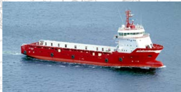
Mid 90s First UT 755 Platform supply (Most common PSV design. Pictured is Dina Merkure , built in 2006)
