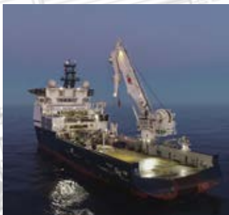
UT 797 CX Anchor handler Island Victory World record bollard pull (477 tonnes)
