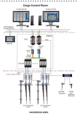
Figure 9: Single radar configuration (example)
