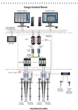
Figure 10: "4-in-2" Dual radar configuration (example)
