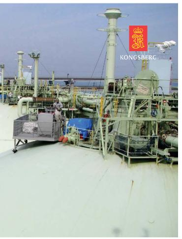
The radar level gauges require no active elements inside the tanks, and with no moving parts the risk for any float trap or tape cutting is eliminated. The powerful radar processing also facilitates for level filtering functions required for ship-to-ship transfer.
