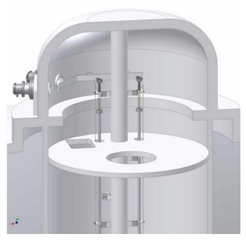
Figure 7: Tank installation, using existing penetration in tank dome (example)
